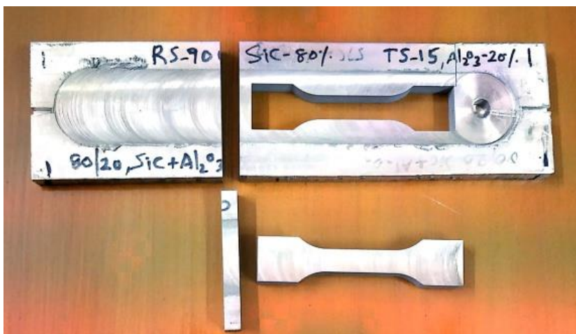
Fig. 2. Image of the Tensile Specimen Processed through EDM.
