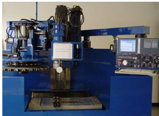
Fig. 1. CNC-Controlled Friction Stir Welding with 2-D welding capability
