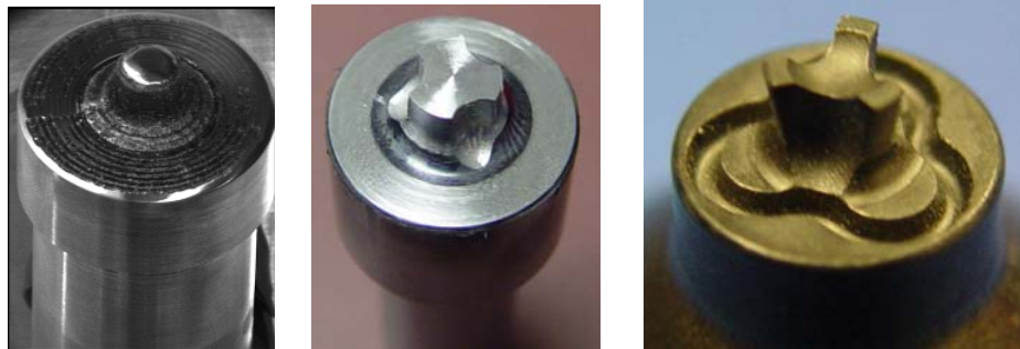
Fig. 5. A few of the tools developed and used for FSW at RCAM
