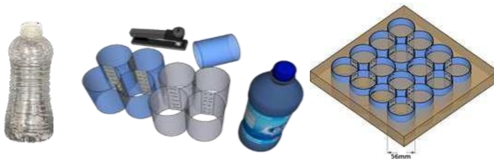
Fig. 4. Assembled bottle mattress to a reinforcement mattress
