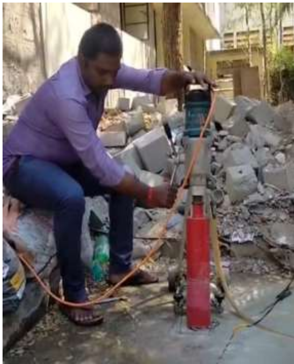
Figure 6: Concrete Core Test
