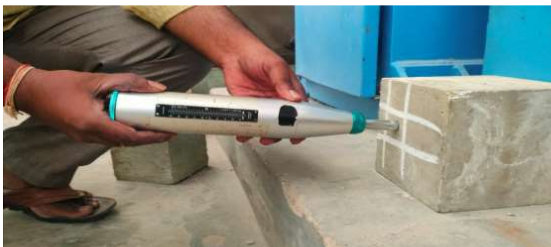
Figure 8: Rebound Hammer Test
