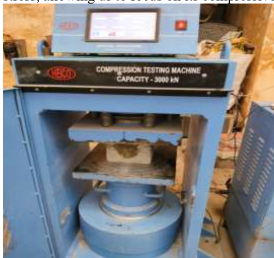
Figure 5: Test for Compressive Strength
