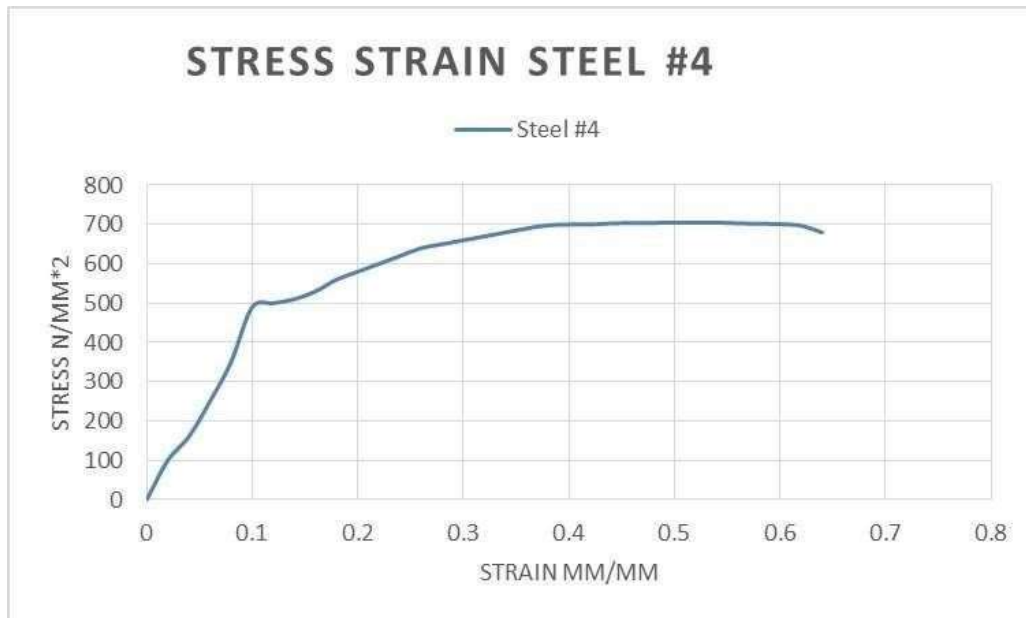
Figure: Shows the Stress-Strain Curves of Steel Bars
