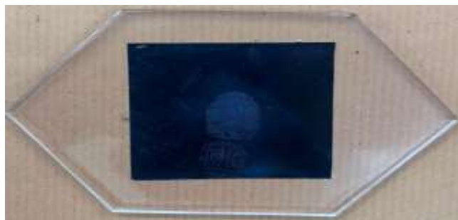
Figure 1. Lifted and preserved powder developed fingerprints using BADGE based resin.
