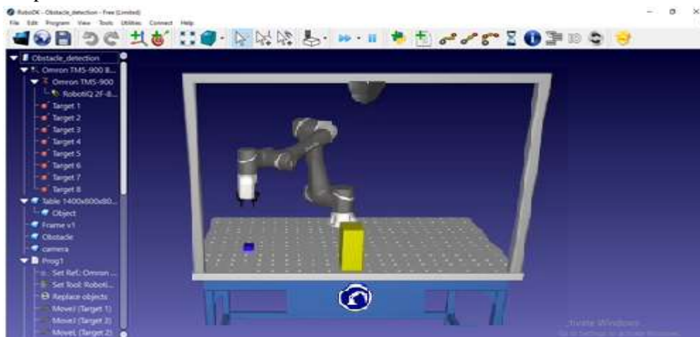
Figure 8. Simulation of pick and place operation of TM5-900
