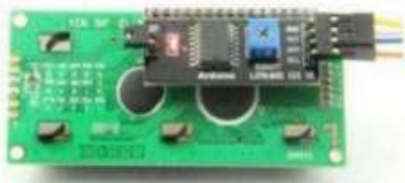
Figure 14. Mounting the I2C Module with the LCD display , .LCD
