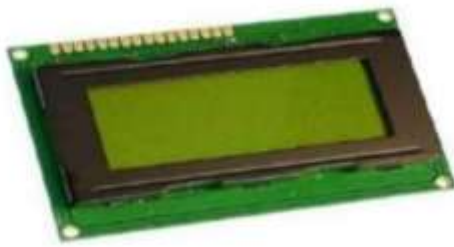
Figure 12 Alphanumeric LCD displays with parallel interface
