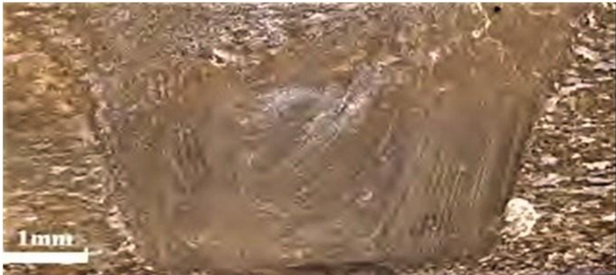
Figure 4. c-s of a weld with alternating bands distributed over the entire bottom
