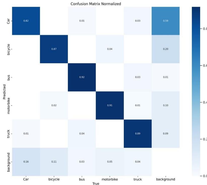
Figure 8: Normalized confusion matrix showing YOLOv8 model's classification accuracy across object categories.
