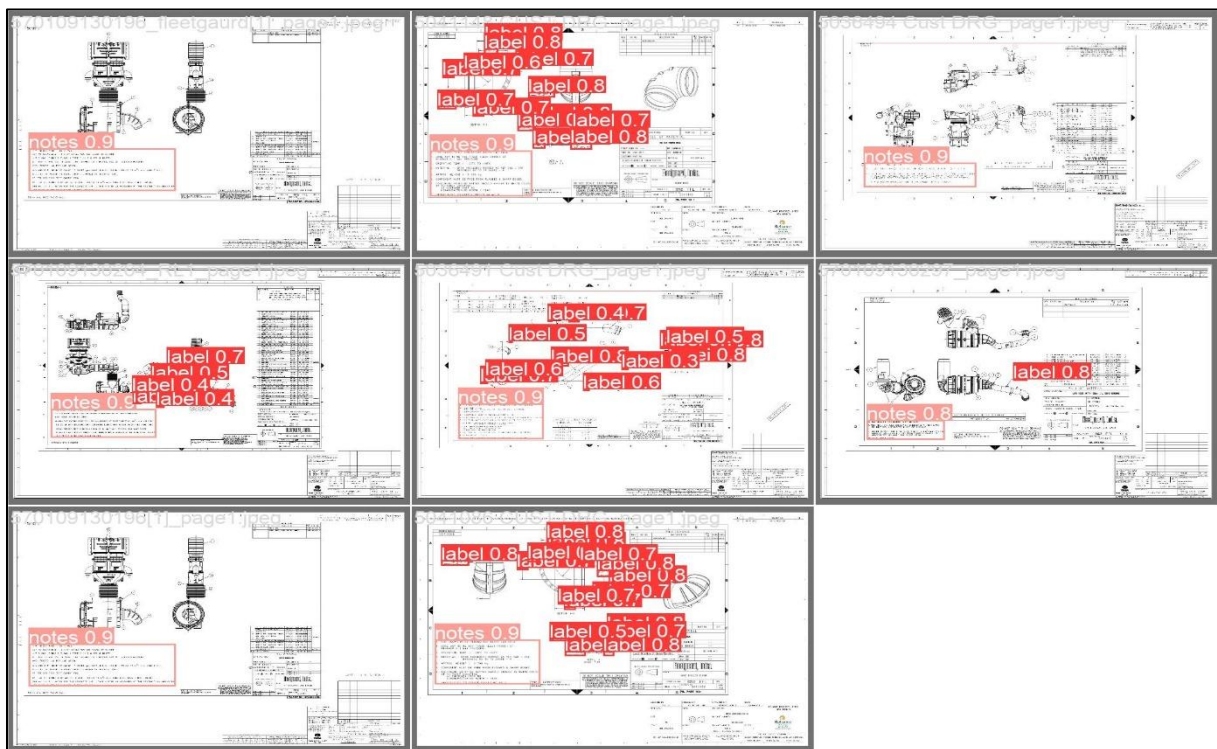
Figure 10. The validation output of yolov8m after 100 epochs ,trained on 2 classes- label (Dimensions) and Notes
