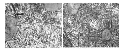
Sample 1(100X) processed at 250°C, 1hr Sample 2(100X) processed at 250°C, 2hr
