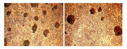
Sample 3(100X) processed at 350°C, 1hr Sample 4(100X) processed at 350°C, 2hr
