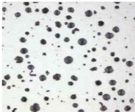
Figure 5 EDX the ductile iron microstructure. Scale bar = 50 \mu\text{m}
