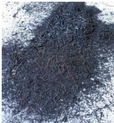
Figure 9. Coil Wires in Residue of Holding Time 15 mn
