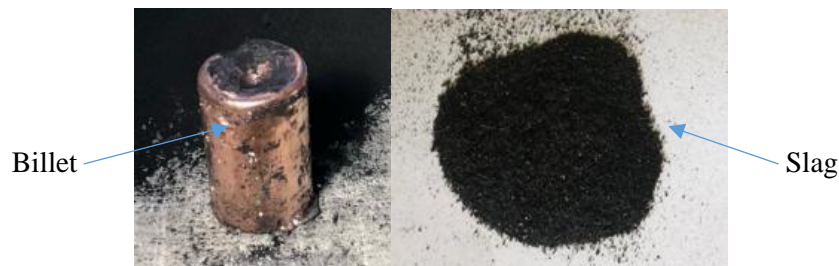
Figure.2 Products of sample melting
